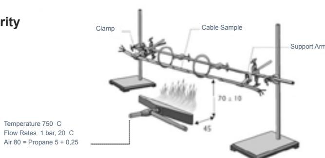
**IEC 60332/1** Fire test on a vertical laid single cable. Test chamber
